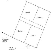
Figure 16. Illustration of Building North Axis
