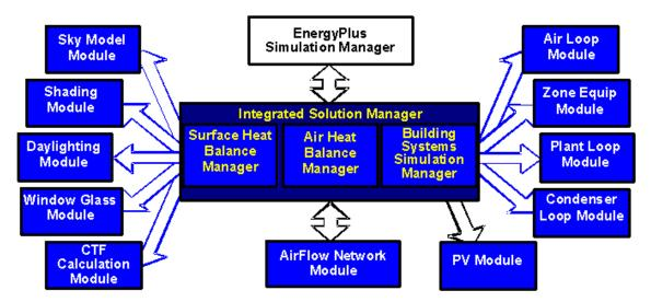
Figure 2. EnergyPlus -- Internal elements
